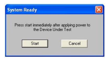
As for the Fluctuating Harmonics test, ensure that the Mains supply is connected to the Product Under Test at the first display and click on the OK button. At the second display, ensure that the Product Under Test is switched on and has settled into steady state operation, and then click on the Start button.
