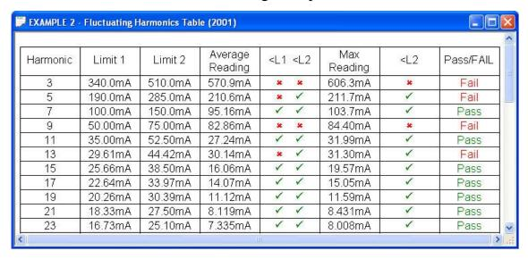
In the example above, the results for harmonic 5 show that the average result has exceeded limit 1 but not limit 2 and that the maximum reading has not exceeded limit 2 resulting in a FAIL for harmonic 5. See the reference information for more details.
