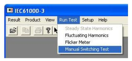
During the test the software automatically displays an ON prompt soon after the beginning of a one-minute test period and an OFF prompt before the end of a one-minute period.
